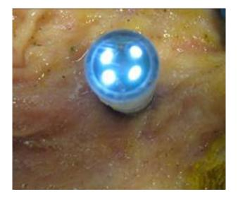
Fig. 7 Wireless illumination module anchored on the gastric mucosa
