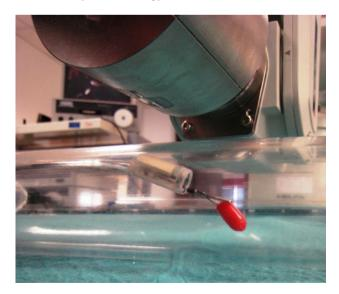
**Fig. 3** View of the MAC inside a transparent plastic tube holding a red object with a standard endoscopic grasper. The MAC is magnetically linked to the external magnet mounted as end-effector of the robotic manipulator
