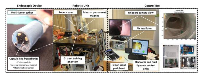
Fig. 1 View of the complete endoscopic platform, consisting of the endoscopic device (left), the robotic unit (center), and the control box (right)
