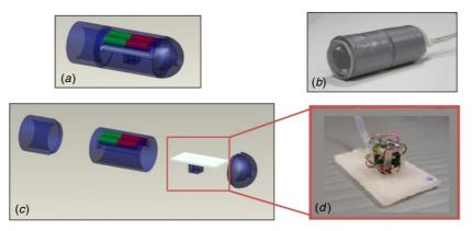
**Figure 5.** (a) The assembled model of the endoscopic capsule, (b) the capsule prototype, (c) the exploded capsule model and (d) the custom triaxial sensor.
