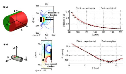
**Figure 4.** EPM in the upper line, IPM in the lower. From left to right: reference system, relative position between the sensor and the magnet with the measuring line and moving direction superimposed to the magnetic field map, comparison between experimental measurements (black dots), measurement uncertainty (black dashed line) and analytical model (red line).
