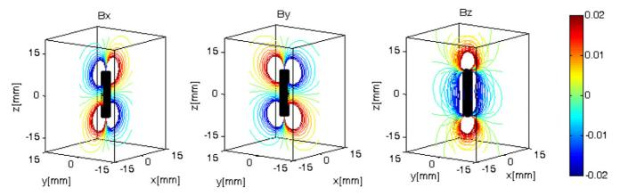
**Figure 3.** IPM magnetic field model solution used to minimize the IPM effect on sensors. Left: axially magnetized single column solution, contour of the magnetic field X component in the Y = 0 plane. Center: contour of the magnetic field Y component in the X = 0 plane. Right: contour of the magnetic field Z component in the X = 0 and Y = 0 planes, color bar in tesla.
