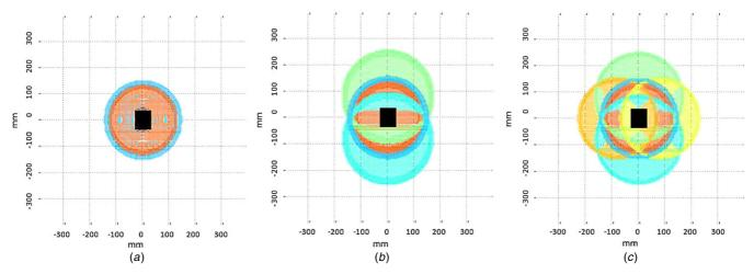
**Figure 8.** Intersection of the calculated iso-magnetic field module clouds of points for defining the XYZ position of the capsule with respect to the EPM. (a) First two measurements above the umbilical region along the Z axis, (b) second two measurements along the X axis and (c) last two measurements along the Y axis.
