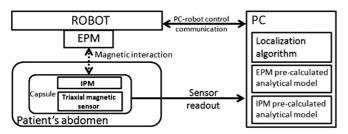
**Figure 1.** Diagram of the platform components involved in the localization procedure.
