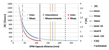
Figure 10. Plot of the magnetic field module and attraction force with respect to the EPM-capsule distance with operating ranges.
