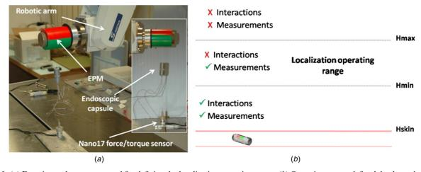
**Figure 6.** (a) Experimental set-up arranged for defining the localization operating range. (b) Operating ranges defined thanks to the test bench.
