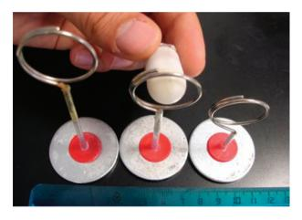
Figure 8. Detail of the ring-shaped targets and comparison with the capsule.
