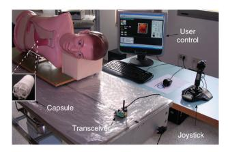
Figure 2. The external unit of the system and the endoscopic capsule located in an upper torso simulator.
