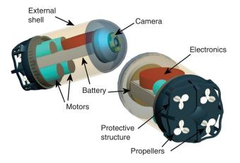
Figure 3. 3D sketch of the capsule and its internal components.
