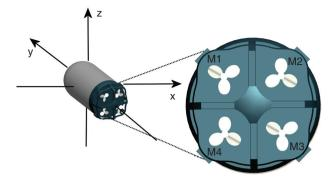
Figure 1. Schematic representation of the capsule and its four propellers.
