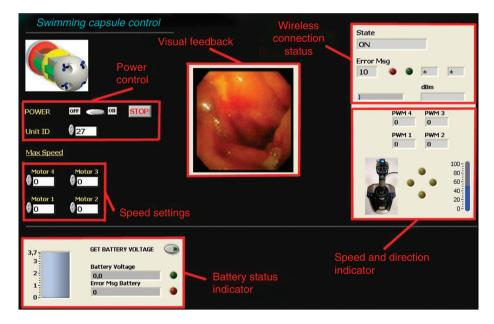
Figure 6. Screenshot of the graphical HMI with descriptions of its different parts.
