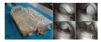
Fig. 15. (a) Ex vivo bench test. (b)–(d) Activation of the legged mechanism to get rid of collapsed tissue. (e) Magnetic locomotion starts again after removing the tissue around the capsule.
