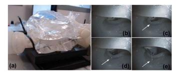
Fig. 14. (a) *In vitro* bench test. (b) Capsule is stuck in the cavity. (c)–(e) Activation of the legged mechanism to get rid of collapsed lumen (see white arrow).
