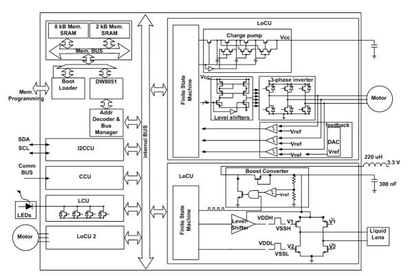
Fig.4: Architecture of the SoC and detail of the motor and lens drivers.
