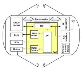
Fig. 2: System architecture of the capsule.
