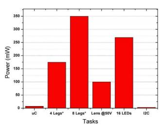
\*Measurements have been done during the stationary phase. Fig.5: Measured power consumption.
