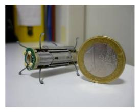
Fig. 1: Capsule without plastic cover. The capsule is equipped with legged locomotion and illumination. Capsule size is 10mm x 33mm.
