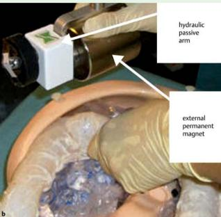
**Fig. 3** a The lower gastrointestinal tract phantom set-up. **b** The phantom set-up and the external magnet on the hydraulic arm.
