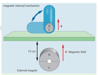
**Fig. 2** The working principle of the magnetic internal mechanism (MIM) capsule. When the motor is activated, the capsule rotates as the intracapsular magnets stay in the same position with respect to the external magnet.
