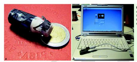
**Fig. 1 a** The clipping capsule loaded with the over-the-scope clip (OTSC). **b** The human-machine interface (HMI) is a personal computer. The USB transceiver (bottom left corner) allows wireless communication with the capsule.
