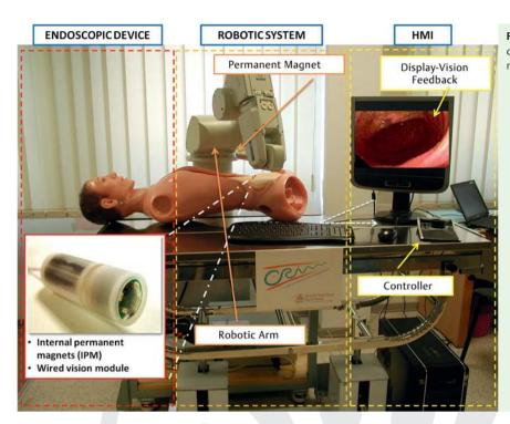
**Fig. 1** System architecture of the robotic platform composed of a human-machine interface (HMI), the robotic system and the endoscopic capsular device.
